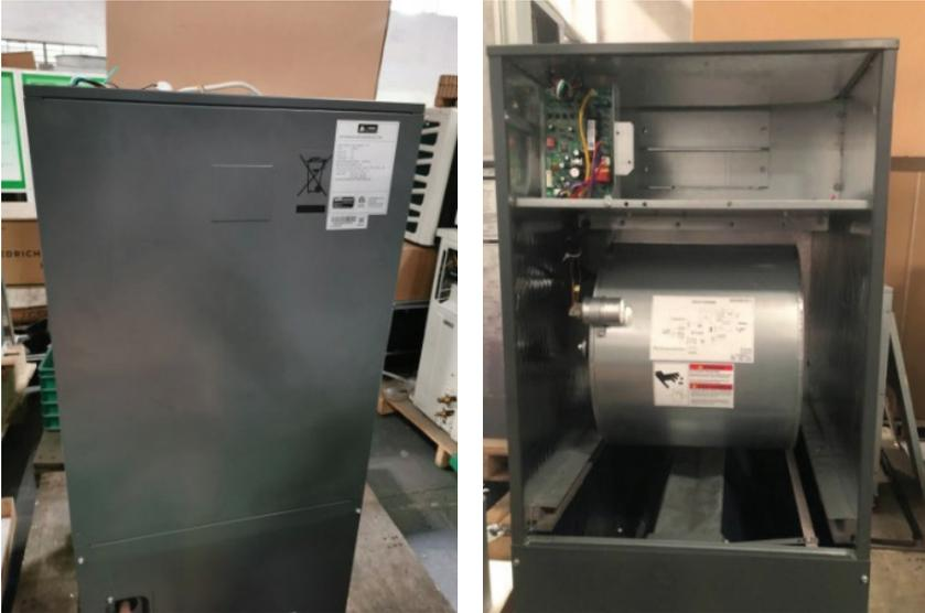
2.) Remove the air duct sealing plate by removing the 4 screws
