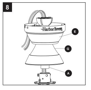
Slide the downrod (A) into the yoke of the motor assembly (H), align the holes, then re-install the downrod pin (B) and downrod clip (C). Secure with set screws (I) and slide the yoke cover (G) down until it rests on top of the motor assembly (H).
