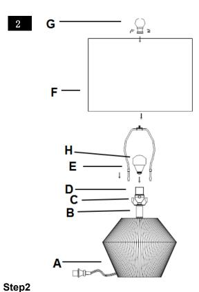
Insert the Harp (E) into the Saddle (C). Put the shade(F) on the Harp(E), then tighten the Finial (G)into the Harp (E) Insert the bulb(H) into the socket(D).
