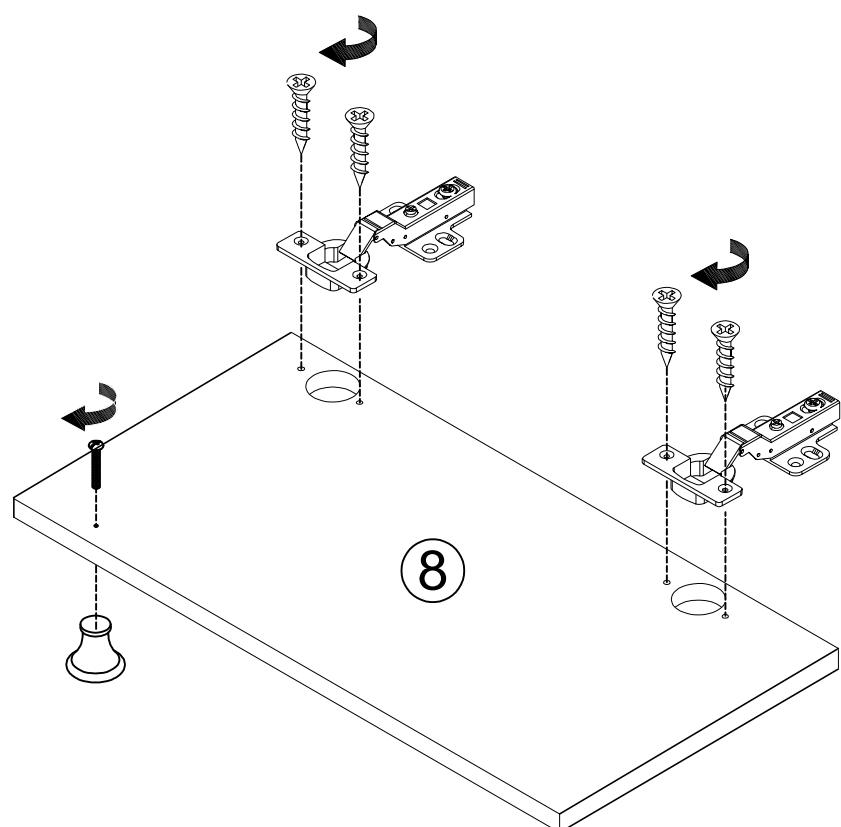
◦ Use Screws to install the handle and apply Screws to fix the hinge on the door #8 and #9
