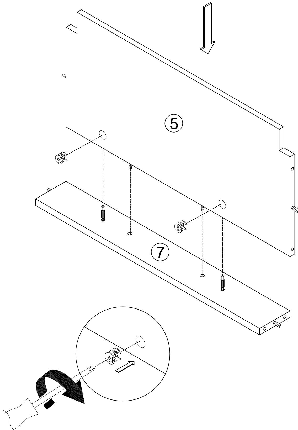
° Refer to the illustration, already assembled #7 on the shelf #5. Then tighten the cam lock
