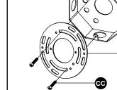
4. Align the 2 screws(AA) through the holes of the back plate, and fix them with screw nuts.
