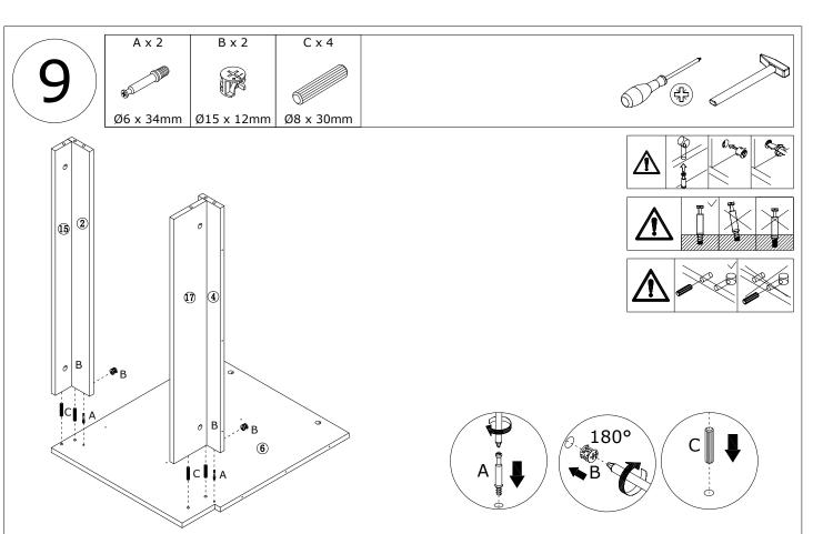
Insert quickfit screw(A) into part 6. Hammer one wooden pin(C) into part 2&15 and part 4&17 respectively. Attach two components to part 6, turn cam locks(B) clockwise to tighten as shown.
