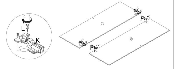
Fix hinge(K) to part 31 another part 30 with screw(L) as shown.
