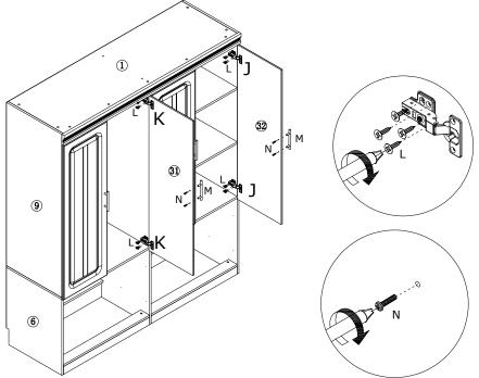
Attach part 32 to part 10, fixing hinge(J) with screw(L) as shown. Fix handle(M) to part 32 with screw(N) as shown. Attach part 31 to part 11, fixing hinge(K) with screw(L) as shown. Fix handle(M) to part 31 with screw(N) as shown.
