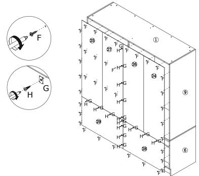
Cover part 24, 25, 26, 27, 28 and 29 to the unit with screw (F). And use part (G) and (H) to reinforce each panel.
