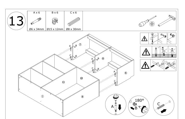
Insert quickfit screw(A) into part 12. Connect 2 components with wooden pin(C), turn cam locks(B) clockwise to tighten as shown.
