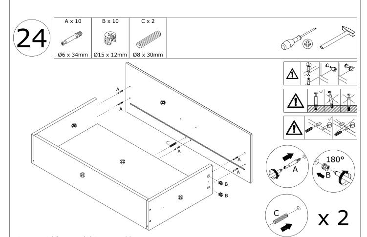
Insert quickfit screw(A) into part 33. Attach part 33 to assmebled unit with wooden pin(C), turn cam locks(B) clockwise to tighten as shown.
