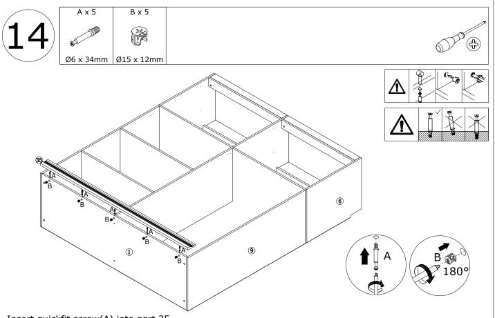
Insert quickfit screw(A) into part 35. Attach part 35 to part 1 with wooden pin(C), turn cam locks(B) clockwise to tighten as shown.
