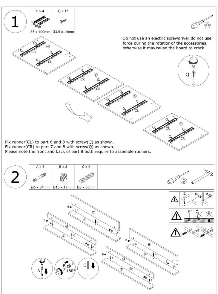
Insert quickfit screw(A) into part 2, 3, 4 and 5. Hammer wooden pin(C) into part 15, 16, 17 and 18. Attach these parts respectively, turn cam locks(B) clockwise to tighten as shown.
