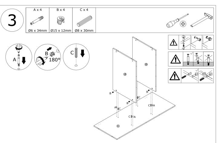
Insert quickfit screw(A) into part 11. Attach two part 13 to part 11 with wooden pin(C), turn cam locks(B) clockwise to tighten as shown.
