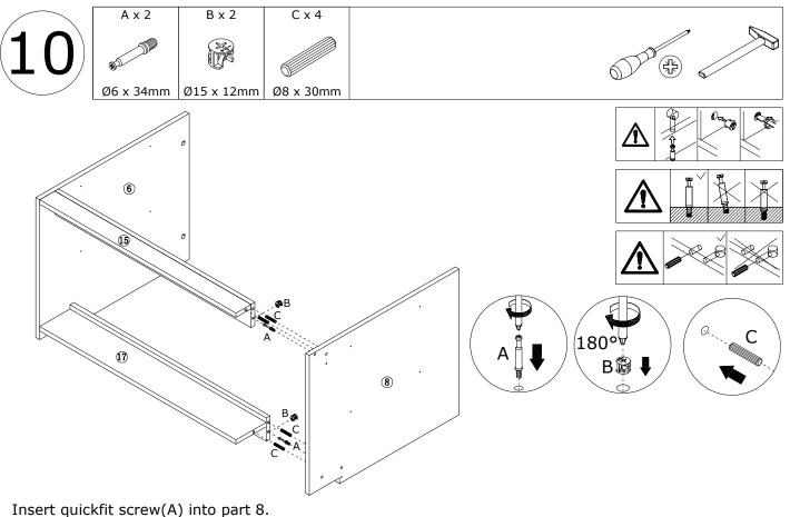
Attach part 8 to assmebled unit with wooden pin(C), turn cam locks(B) clockwise to tighten as shown.
