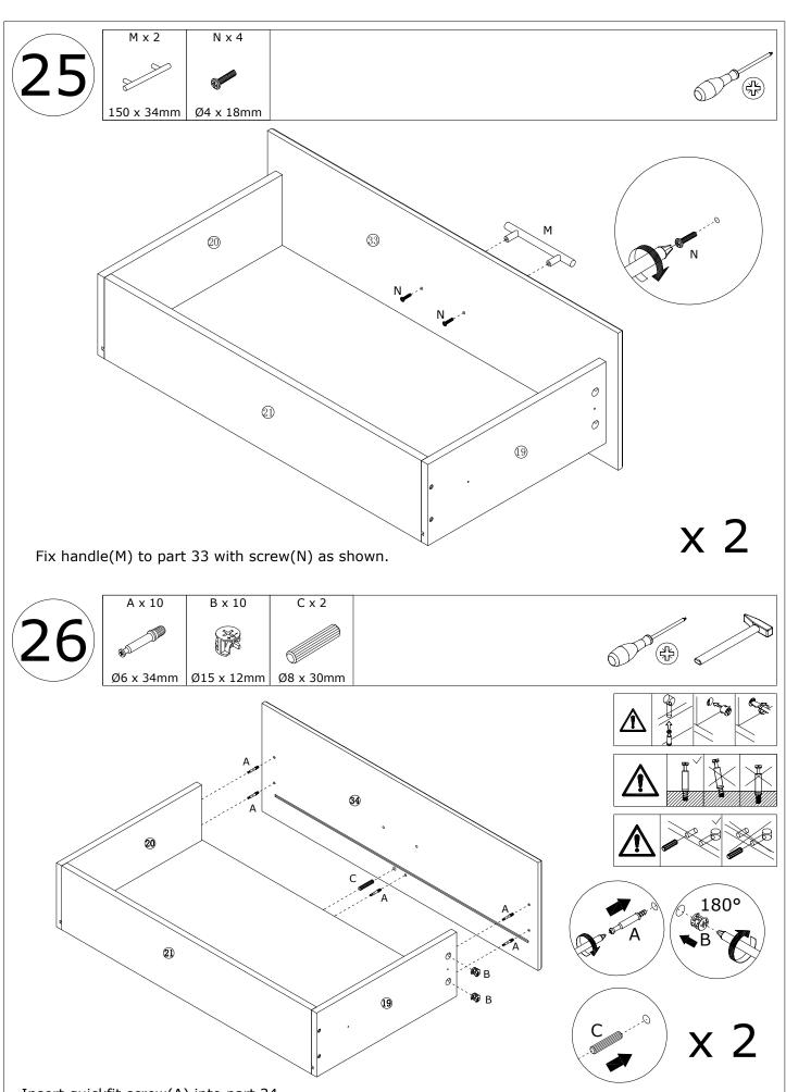
Insert quickfit screw(A) into part 34. Attach part 34 to assmebled unit with wooden pin(C), turn cam locks(B) clockwise to tighten as shown.
