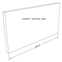
Measure the length (in feet) of each wall being covered.
