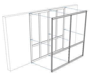
Install vinyl rail extrusions over the polystyrene strips using construction adhesive. Use 5/8" flat head screws to secure rails until adhesive cures.
