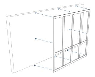
Mount polystyrene strips directly to masonry walls or drywall using construction adhesive at the bottom of the drop ceiling, base of walls, every two feet on center and along the chair rail.
