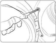
3. Remove the two screws on the opposite side of the door hinge.
