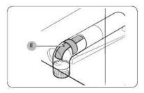
Apply duct tape (E) on the joint as shown.
