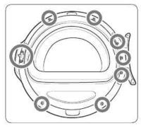
Locate and remove the 9 screws from the door as shown.
