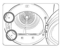
**13.** Insert and tighten the two screws on the opposite side of the door hinge.
