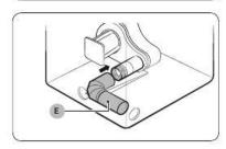
Insert the duct with elbow (E) through the rear opening, and then connect it to the internal duct.
