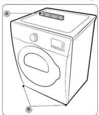
Using a level (A), check if the dryer is level side to side and then front to back. If the dryer is not level, adjust the leveling feet (B) at the bottom of the dryer. Then, check if the dryer is level again.
