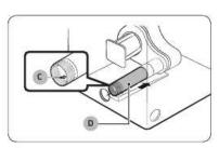
Reconnect the cut portion of the duct (D), and then fasten it to the ramp on the appliance base with the screw (C) which you set aside in Step 2.
