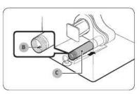
Reconnect the cut portion of the duct (C), and then fasten it to the ramp on the appliance base with the screw (B) which you set aside in Step 2.
