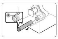
Pull the duct out of the dryer, and then remove the screw (B) from the duct. Set screw (B) aside. You will need it in a later step.
