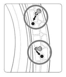
Move the location of the screws, used to fix the door hinge, as shown.
