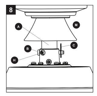
9. Depending on the length of downrod you use, you may need to cut the lead wires back to simplify the wiring. If you decide to cut back the lead wires, take the lead wires and make sure you have pulled them all the way through the top of the downrod. Measure at least 8 inches of lead wire, then cut the excess wire off with wire cutters (not included).
