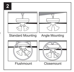
3. Ensure the blades (R) will be at least 30 in. from any obstructions. Also check the downrod (A) length to ensure the blades (R) will be at least 7 ft. above the floor.
