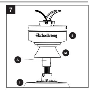
8. Slide the downrod (A) into the yoke of the motor assembly (I), align the holes, then re-install the downrod pin (B) and downrod clip (C). Secure with the two set screws (H) and slide the yoke cover (M) down until it rests on top of the motor assembly (I).
