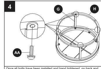
Once all bolts have been installed and hand tightened, go back and tighten firmly with wrench (BB).
