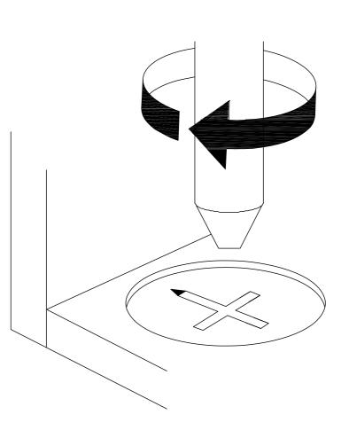
Turn cam lock clockwise to tighten.
