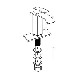
**7.** Screw the water inlet hose nut onto the water valve and tighten it with a wrench. Finally, open the water valve and enjoy your waterfall.
