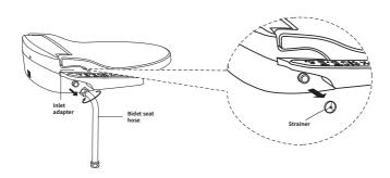
4. AFTER ATTACHING THE HOSE TO THE INLET ADAPTER, TURN THE WATER SUPPLY VALVE TO THE LEFT AND HAVE IT OPENED.
