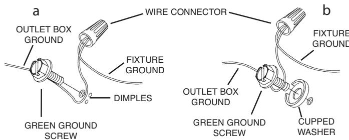
4. Make wire connections. Reference chart below for correct connections and wire accordingly.
