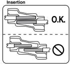
In order to remove solid conductors, pull and twist back and forth. For stranded wire, use a new connector.
