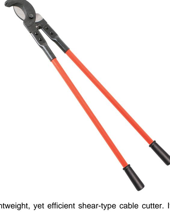
Klein Tools' Communication Cable Cutter is a lightweight, yet efficient shear-type cable cutter. It is designed to cut up to 900-pair soft copper and aluminum cable, and also lead or rubber-covered communications cable. Forged steel jaws make a clean, even cut for ease in fitting lugs and terminals.
