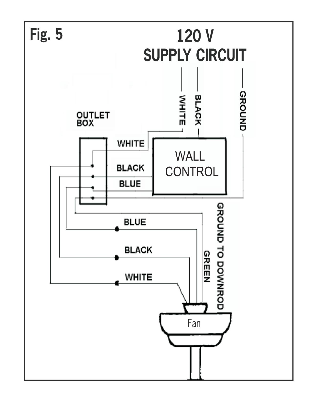
**NOTE:** Once ground wires are connected, carefully tuck all wires and marrettes into the metal outlet box making sure that the wires are clear of the hemisphere and downrod when positioned in mounting bracket.
