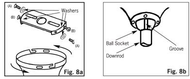
**NOTE:** When installing fan on sloped ceiling, make sure tab on hanger bracket faces towards the top of the slope. Depending on the slope, a longer downrod may be required to prevent fan blades from hitting the ceiling.
