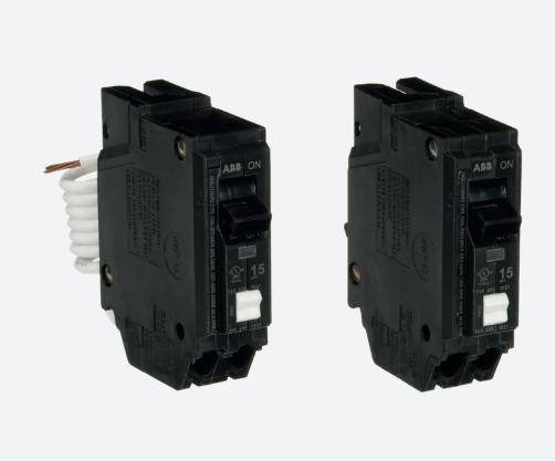
An Arc Fault Circuit Interrupter (AFCI) detects arc faults and de-energizes the circuit to prevent electrical fires. Combination arc fault circuit interrupters protect against overloads, short circuits, parallel arcs, and series arcs. Combination AFCI comply with the 2008 and forward National Electric Code (NEC) requirements for dwelling units.
