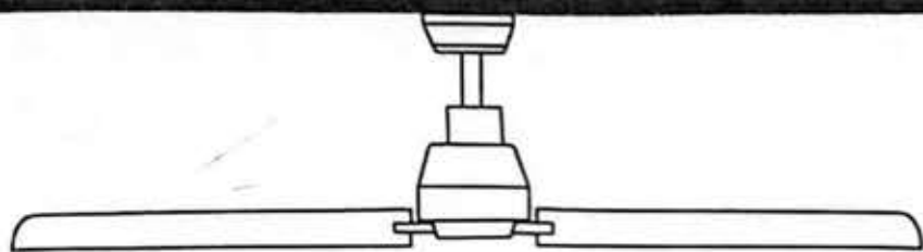
Horizontal ceiling installation
