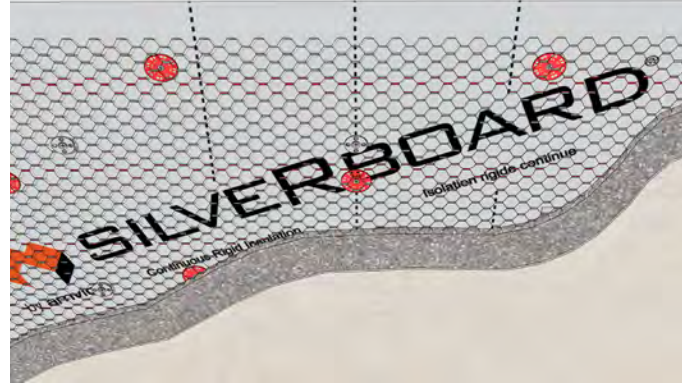
Figure 32 – Synthetic stucco with 2" (51mm) high density SilverBoard installed with drainage cavity method 2
