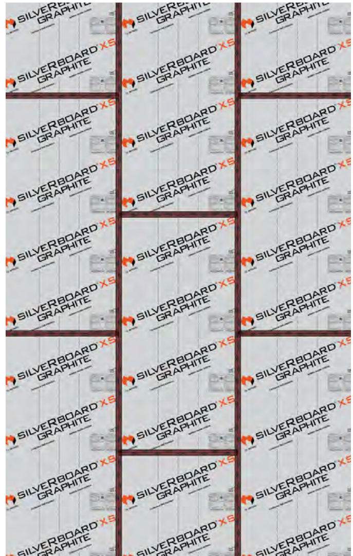
Figure 17 – Taping pattern for vertical board orientation
