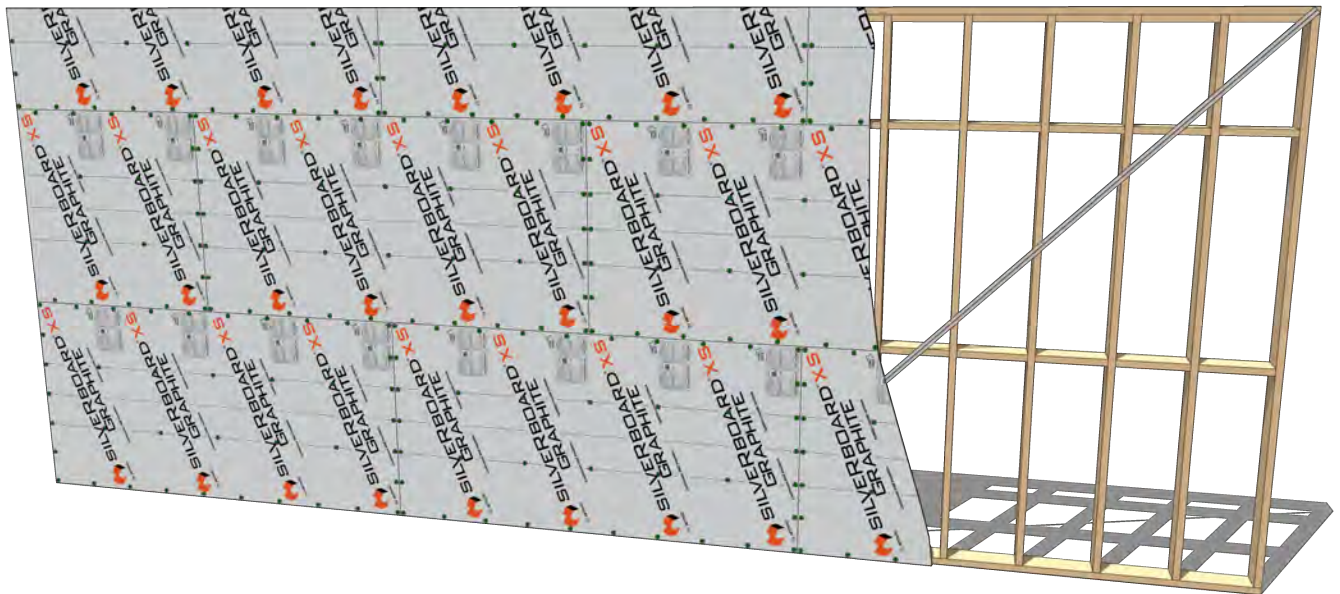
Figure 4 – Horizontal SilverBoard installation over open stud wall assembly
