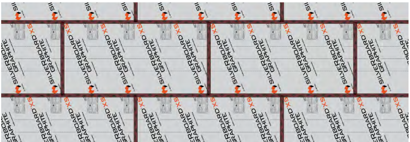
Figure 18 – Taping pattern for horizontal board orientation
