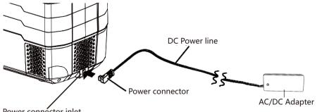
Plug the AC power line into the wall socket (AC 100-240V,50/60Hz)
