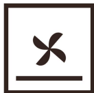
Fan and bottom heater on
