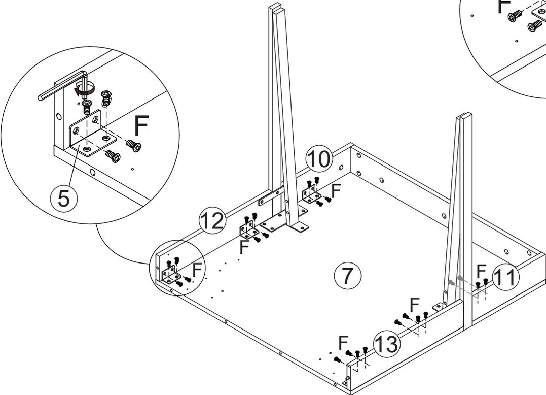
Fix iron sheet 5 to board 7, 10, 12, 11 and 13 with screw(F) as shown.
