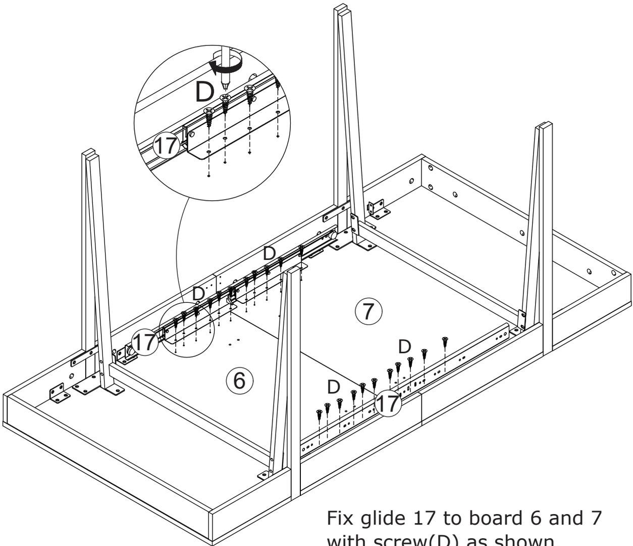
Fix glide 17 to board 6 and 7 with screw(D) as shown.
