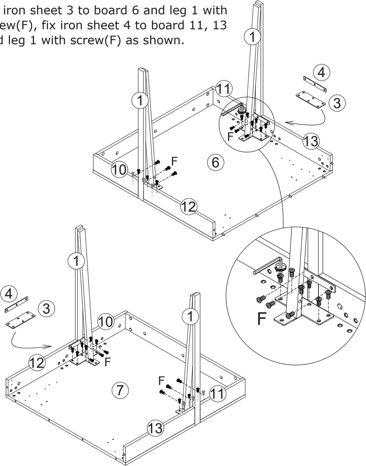
Fix iron sheet 3 to board 7 and leg 1 with screw(F), fix iron sheet 4 to board 10, 12 and leg 1 with screw(F) as shown.
