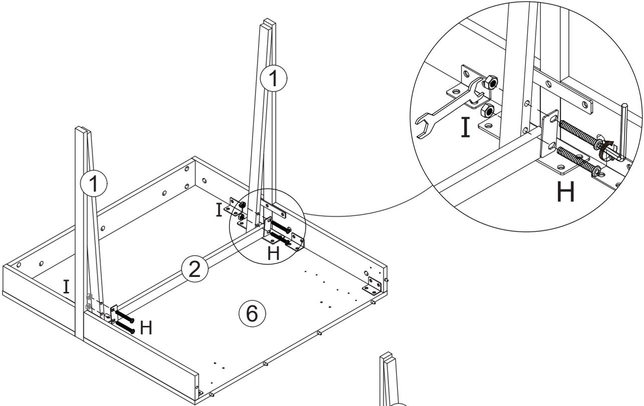
Fix steel tube 2 to leg 1 with screw(H) and nut(I) as shown.
