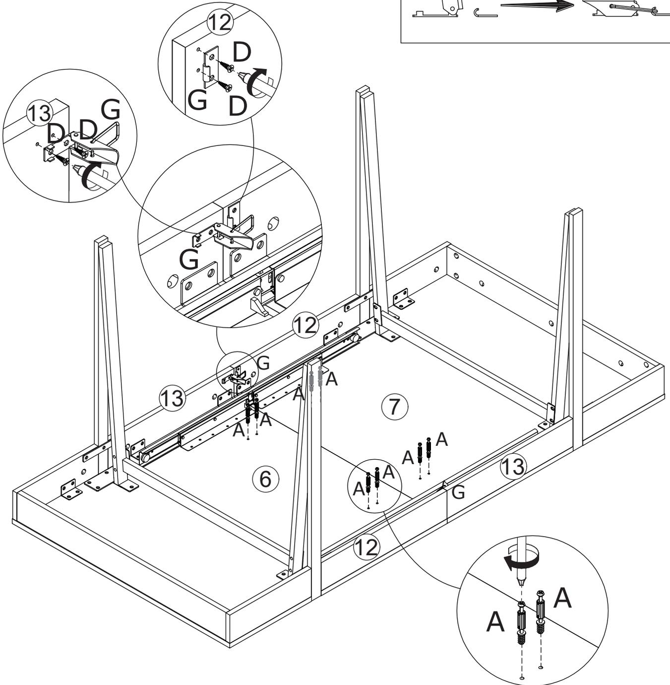
Screw eccentric rod(A) into board 6 and 7 with a screwdriver as shown.
