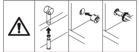
Attach board 15 to board 6 and 7, add cam lock(B) into board 15 and turn clockwise to tighten as shown.
