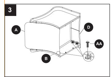
Hand tighten AA. Do not tighten until all bolts have been installed.
