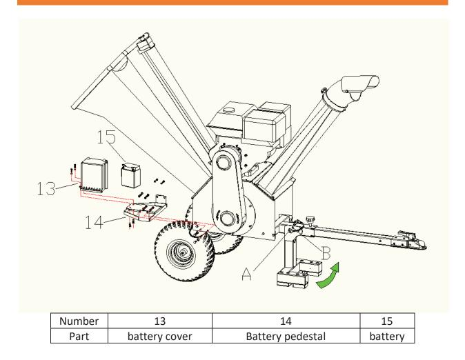
13. Battery into battery cover first then slide onto battery pedestal under feed chute.
