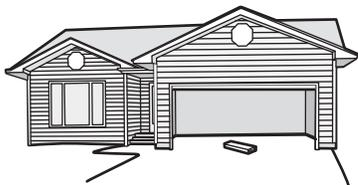
2 Press the remote control push button to close the door. The door **MUST** reverse when it makes contact with the board.
