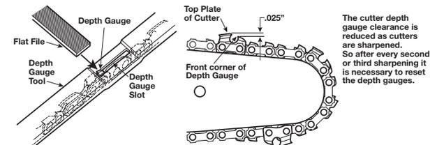
The cutter depth gauge clearance is reduced as cutters are sharpened. So after every second or third sharpening it is necessary to reset the depth gauges.
