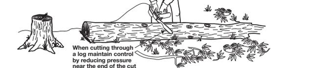
Fig. 12 Bucking a Log when its Entire Length is Resting on the Ground
