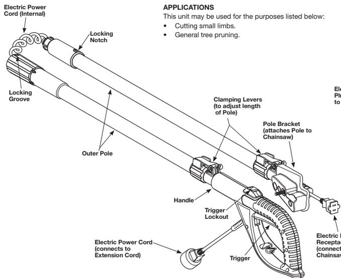
Fig. 2 Remington RM1015SPS Telescoping Pole Assembly
