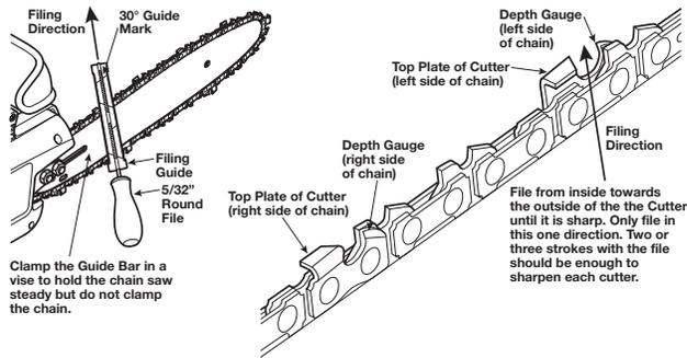
**Items Needed to Sharpen Chain Saw Cutter Teeth**
