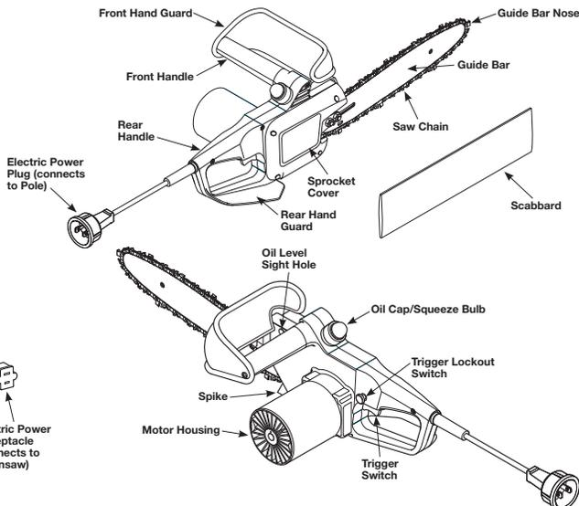
Fig. 3 Remington RM1015SPS Chainsaw (Right and Left Sides)
