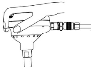
4. Align fastener and tool in the location where fastener is to be driven.
