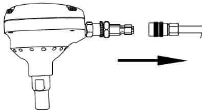
2. Turn the tool so the air inlet is facing up. Place 2-3 drops of pneumatic fastening tool oil into air inlet. Do not use detergent oils, oil additives, or air-tool oils. Do not use detergent oil or additives as these lubricants will cause accelerated wear to the seals and bumpers in the tool, resulting in poor tool performance and frequent tool maintenance.
