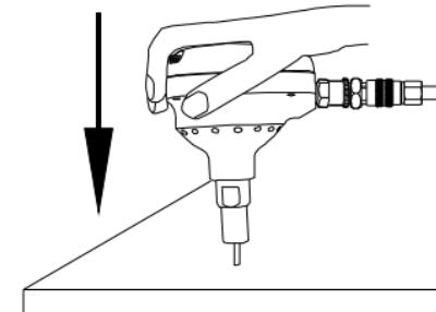
6. Continue to apply pressure until fastener is driven completely or until reaching desired penetration.
