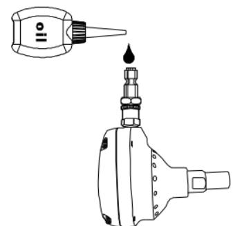
3. After adding oil, run tool briefly. Wipe off any excess oil from the cap exhaust.
