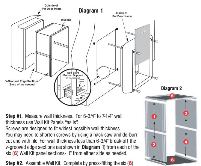
**Step #3.** With a second person holding "OUTSIDE FRAME" of dog door in place, insert assembled Wall Kit into opening from inside. Place "INSIDE FRAME" of dog door into opening around the Wall Kit.
