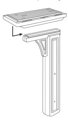
Slide wrap onto base until it snaps into place.
