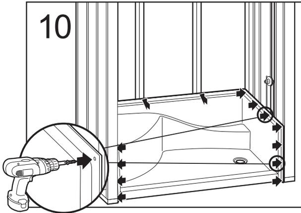
Pre-drill horizontal and vertical flanges and fasten into each corresponding stud.
