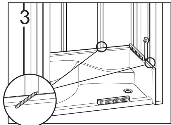
Level and mark all sides. Front apron should be firmly on the floor.
