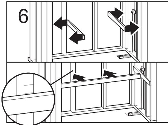
Fasten a wooded 1" x 3" along the rear and sides of framing (immediately below marks).
