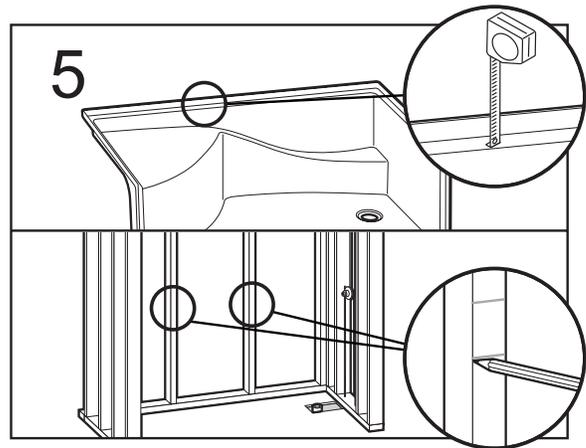
Measure the distance between the top of the back horizontal flange and the bottom of the pan ledge, at approximately 1-1/2". Mark this dimension on the back studs, below the first mark of step 3.
