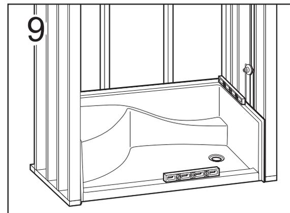
Tap down until level. Level horizontally and vertically using a level. Use shims if necessary. The apron should be resting firmly on the ground.
