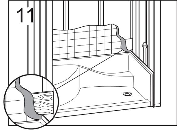
Finishing panels (plasterboard, ceramic tile, etc.) should completely cover the fastening flange. The joint between the wall panels and the finishing panels can be covered with a joint compound, a plastic stripe, or a tile strip.
