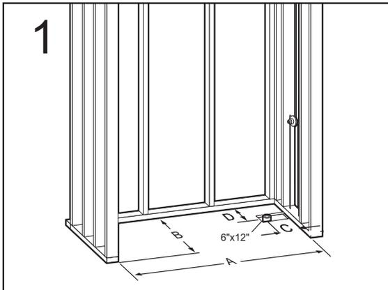
Check dimensions. **NOTE: If you're adding additional accessories such as a grab bar—additional framing or backing may be needed for support.** Pre-install unit to ensure framing pocket is plumb, square, and a level installation can be achieved. (See steps 2 and 3.) Adjust framing as needed – shim where necessary.
