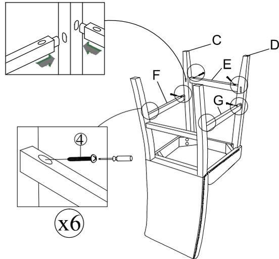
STEP 5: To level the chair, stand the chair up on a flat surface and tighten all the bolts by using Allen Key (7) and all the screws with a screwdriver.
