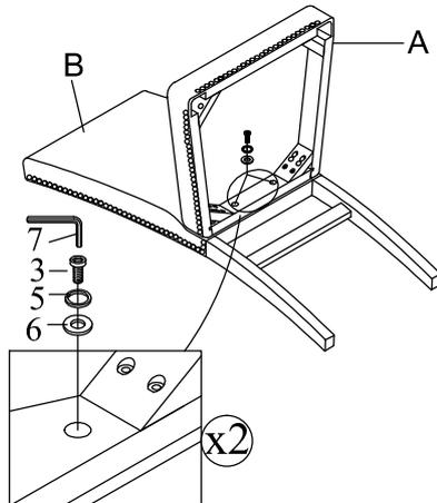
**STEP 2:** Assemble the cushion seat (A) with the back legs of the chairback (B) by using Allen Key (7) with hardware 1, 5, and 6.
