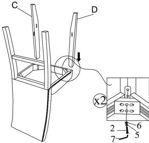
STEP 4: Install the front stretcher (E) between the front legs (C & D), then install the LSF stretcher (F) by inserting the end with the label "front" into the front LSF leg (C) and the RSF stretcher (G) by inserting the end with the label "front" into the front RSF leg (D).
