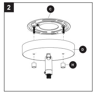
3. Use the bracket screws (RR) to attach the mounting bracket (C) securely to the outlet box (sold separately).
