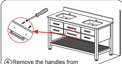
④ Remove the handles from inside the cabinet doors and drawers and reinstall on the outside. Do not over-tighten when reattaching.
