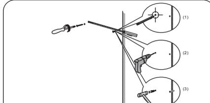
⑤ Install the mirror: use a pencil to mark the placement of the screw holes on the wall, drill the holes and insert the plastic wall anchors.
