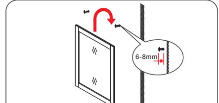
⑥ Install the screws into the wall anchors, leaving enough of the screw exposed to hang the mirror - approx 1/4" - 1/2".
