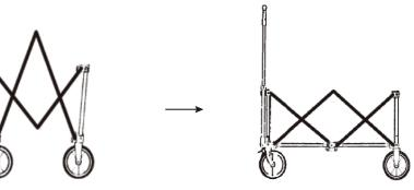
2.**Folding and storing:** After taking out the folding bottom plate, gently lift the bottom center pull ring, and the frame will automatically collapse.
