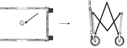
3. When not in use, press and hold the middle button on the pull rod to shorten the pull rod. When in use, directly pull out the pull rod. The pull rod can be positioned within 90 degrees and can be subjected to forces used by people of different heights.
