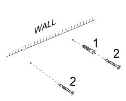
Note: No drilled hole or plastic anchor required when mounting to stud or wood wall. Use screw only. We do not supply hardware for mounting on concrete walls. Find a desired location. Mark 2 locations for screws on wall in the same distance as the mounting holes on the back of the unit.
