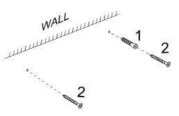
Note: No drilled hole or plastic anchor required when mounting to stud or wood wall. Use screw only. We do not supply hardware for mounting on concrete walls.
