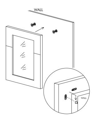
Hang the Wagars Mirror onto the Screw (2) and verify the mirror is resting securely on the mounting Screw (2).
