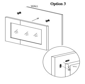
Hang the Wagars Mirror onto the Screw (2) and verify the mirror is resting securely on the mounting Screw (2).
