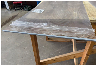
Edge Sealing: Aluminum Solid Tape
