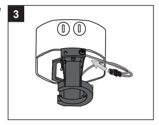
Align the canopy (E) over the loose mounting bracket screws (V) preassembled on mounting bracket (D).
