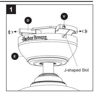
2. Secure the canopy (E) with the mounting bracket screws (V) previously removed (Step 4, page 8). Tighten all mounting bracket screws (V) securely.
