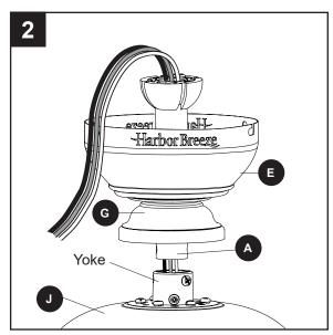
3. Slide the downrod (A) into the yoke of the motor assembly (J), align the holes, then re-install the downrod pin (B) and downrod clip (C). Secure with set screws (K).
