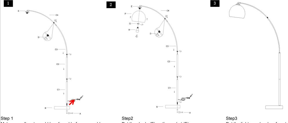
Make sure all parts could be aligned before assemble Do not rotate lamp body too hard avoid base screw broken
