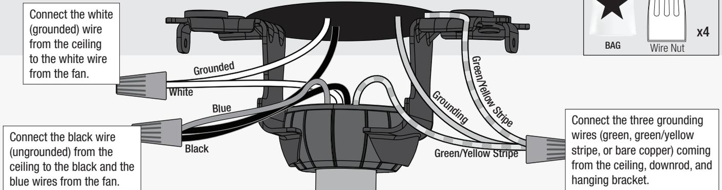
**⚠ WARNING** The ceiling fan must be grounded. If the ground wire for the installation site is not present, immediately **STOP** installation and consult a qualified electrician.
