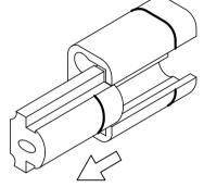
You can pull the buckle out by following the direction indicated by the arrow
