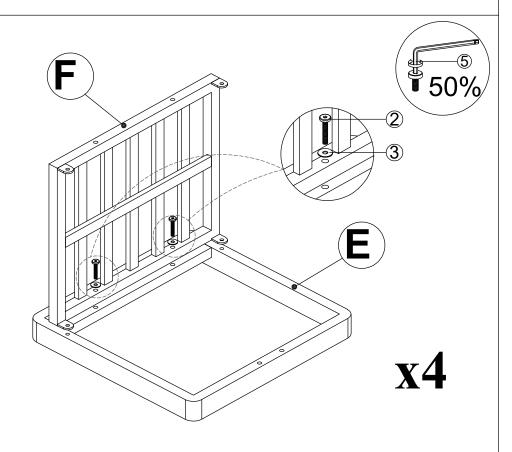
Connect Leg Stool (E) & Seat Stool Frame (F), Tighten Bolt (2) & Flat Washer (3) with Allen Key (5).
