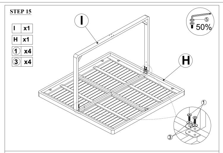
Connect Top Table (H) & Table Leg Middle (I), tighten Bolt (1) & flat washer (3) with Allen Key (5).
