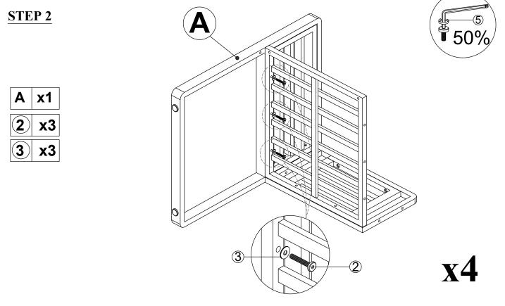
Connect the part from step 1 & Right Leg (A), Tighten Bolt (2) & Flat Washer (3) with Allen Key (5).
