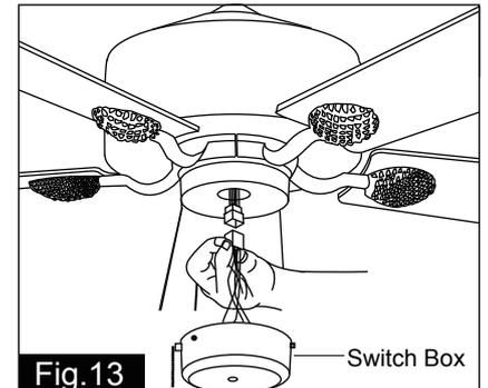
Connect the two terminals respectively from the motor and the switch box.
