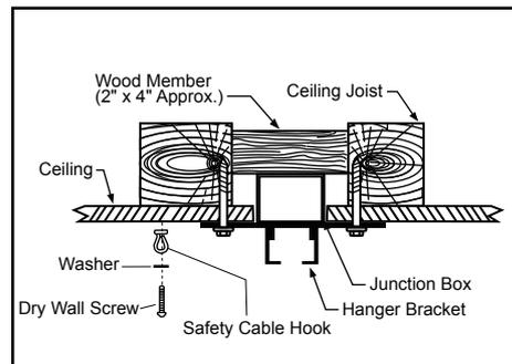
Tighten the hanger bracket to the outlet box with two mounting screws. **(Make sure the outlet box is securely installed so that it will be able to support at least the fan weight.)** Attach the safety cable hook to the ceiling with the dry wall screw and washer, and make sure the safety cable hook is covered by the fan canopy. **WARNING: MOUNT ONLY TO AN OUTLET BOX MARKED "ACCEPTABLE FOR FAN SUPPORT"!**
