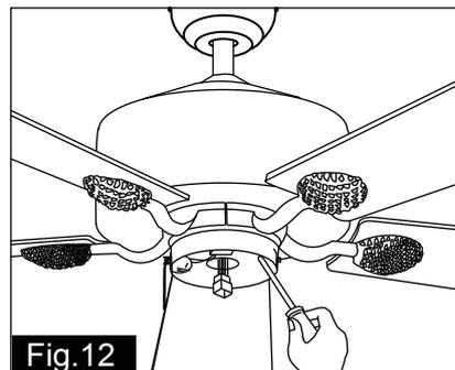
Secure blade brackets to the motor with motor screws and washers.
