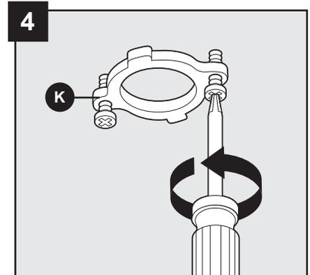
5. Slide rubber washer (I) and metal washer (J) onto shank of faucet body (D). Secure faucet body (D) to sink with lock nut (K) and preassembled screws.
