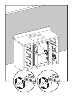
11. To remove drawers preassembled in vanity (A), fully extend drawers. Locate plastic levers on metal glide tracks at left and right sides of drawer box.
