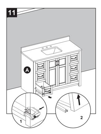
12. To reinstall drawers into vanity (A), fully extend metal glide tracks. Gently lower and slide drawer box into rear glide catch. Next lower drawer box down to completely rest on extended glides. Then, push plastic levers to lock the drawer box in place. Repeat for remaining drawers.
