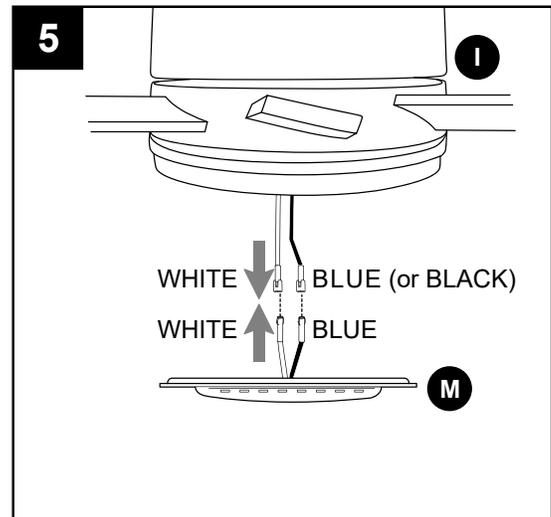
6. Carefully arrange wiring within the fitter plate (J) to ensure wires do not get pinched when attaching the LED light kit (M).
