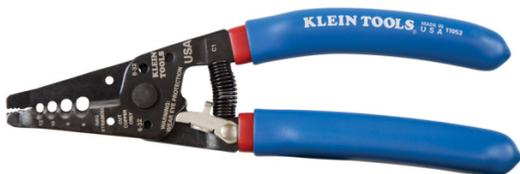
This Klein-Kurve Wire Stripper/Cutter is designed to cut, strip and loop a wide range of stranded copper wires. Precision shear-type blades produce a clean cut. Screw shearing holes cleanly shear 6-32 and 8-32 screws. For use on 6-12 AWG stranded wire.
