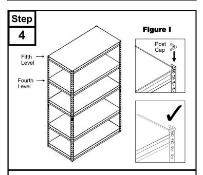
Continue by adding the fourth and fifth level to the unit using two (2) beams and two (2) braces per level. Tap lightly to properly seat the rivets and add the final wood shelves to the unit. Place (4) post caps onto each post (see figure I). Do a final inspection to make sure all rivets are securely seated into the narrow ends of the post slots. The assembly is now complete.
