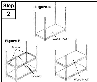
Add a wood shelf to the level previously built (see figure E), then continue working by adding the second level using two (2) beams and two (2) braces in the post slots of your desired location (see figure F). Again, place the rivets of the beams and braces into the post slots with the shelf ledge facing up and tap lightly to seat the rivets. Add a wood shelf to the second level.
