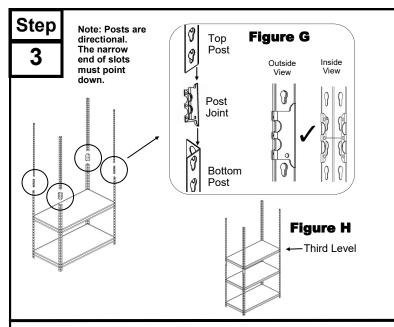
Assemble four (4) posts to the four bottom post assemblies by using four (4) of the post joints. Place the post joint into the top of the bottom post assembly and tap down to properly seat. Next place a post into the top of the post joint and tap down to properly seat (see figure G). Continue by adding the third level using two (2) beams and two (2) braces just above the post joints. Again tap lightly to seat the rivets. Add a wood shelf to the level (see figure H).
