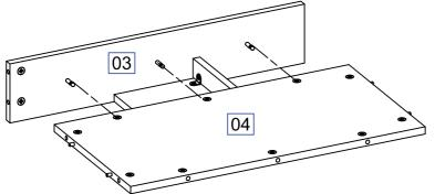
\* Attach part 04 to the part 03 according to the image. Then screw them using the nuts "F".
