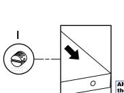
\* Insert hardware "I" on the part 03 and 05. Attention to hole Ø0.47".
