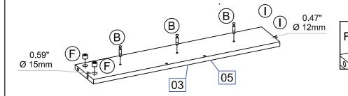
\* Insert hardware "F" on the part 03 and 05. Attention: hole Ø0.59"
