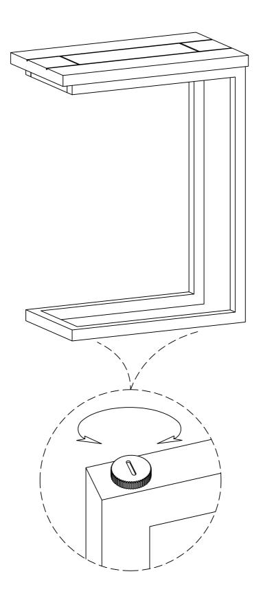
Note: Levelers on bottom of legs can be adjusted if floor is uneven.
